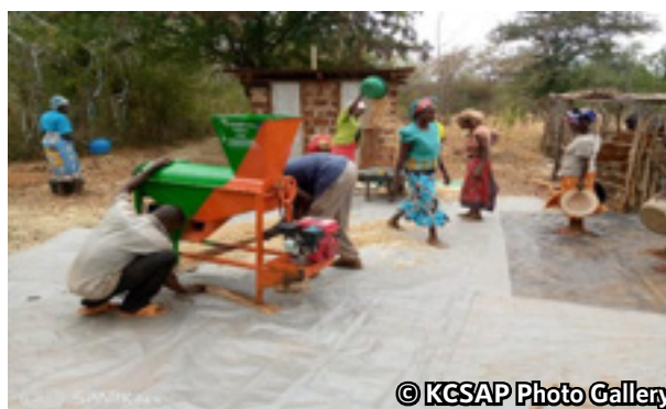
Use of green grams mechanical threshing technology to reduce post-harvest losses
